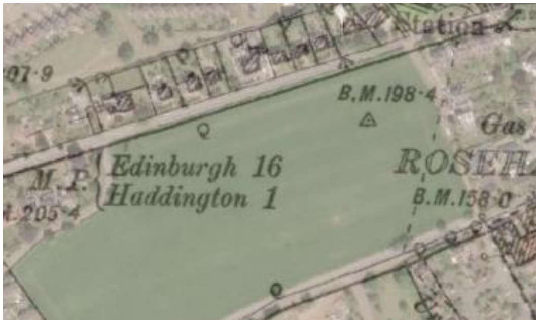
Figure 11 - The OS 6-inch overlay showing a justifiable spot height of 198.4ft at the approximate NE corner of the enclosure
